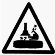
Do not place your hand on the tire. When the hexangular shaft comes back to its work position, the hand between the rim and the tool head may be crushed. Remove the objects may cause the danger to the operators such as bracelet and loose cloth etc. To avoid the accident, when the turntable rotates, you should keep your hand and the other part of your body away from the tool head as far as possible.
