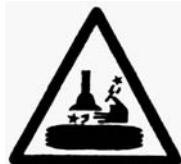
Do not place your hand on the tire. When the hexangular shaft comes back to its work position, the hand between the rim and the tool head may be crushed. Remove the objects may cause the danger to the operators such as bracelet and loose cloth etc. To avoid the accident, when the turntable rotates, you should keep your hand and the other part of your body away from the tool head as far as possible.
