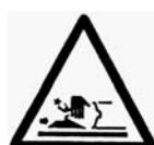
When lock the tire, it is absolutely forbidden to put your hand under the tire. To correctly lock the tire, you should position the tire at the very center of the turntable.
