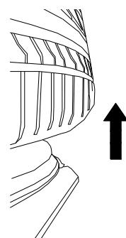
For machines with the assist arm, you can use the tire pressing disk to demount.
