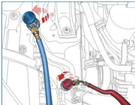
Tighten the A/C system quick-connector counterclockwise
