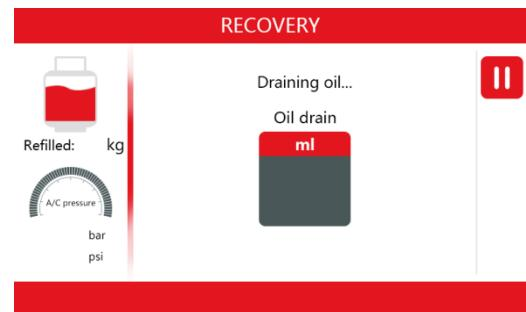
8) Recovery completed. The recovered amount and the oil draining data will be displayed. Press
