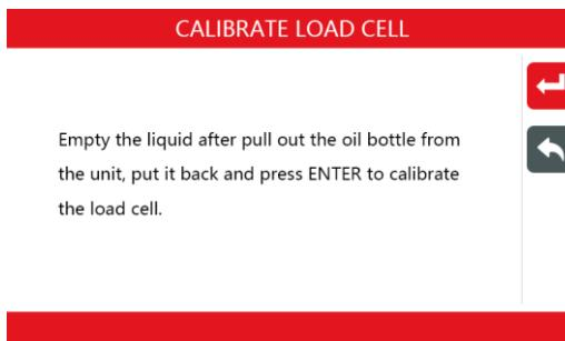
b-2) Please ensure the liquid in the bottle had been emptied, press “Reset” to calibrate the load cell.
