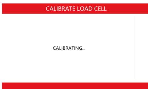
c-4) Calibrate load cell completed. Please take out the weight. Press
