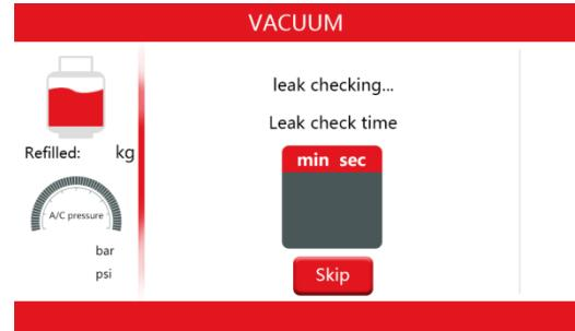
5) Vacuum completed. The vacuum time, leak check time and whether it leak can be observed.
