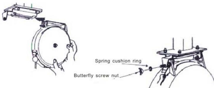
3-4) After fixing the hose reel please join the two terminal of connecting hose separately with "L" connector and braking valve of water pipe.
